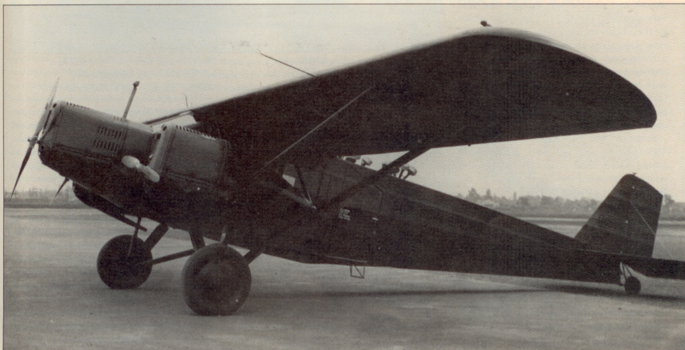
The Ogden Osprey was similar to the structure of single-engine cabin designs of the time. Pilots sat side-by-side and shared a throw-over control column, ahead of a four-seat cabin with a narrow aisle between two rows of seats. A lavatory and baggage compartment were standard features. Aimed at the business aircraft and small airline markets, the Osprey was relegated to other lines of work.
